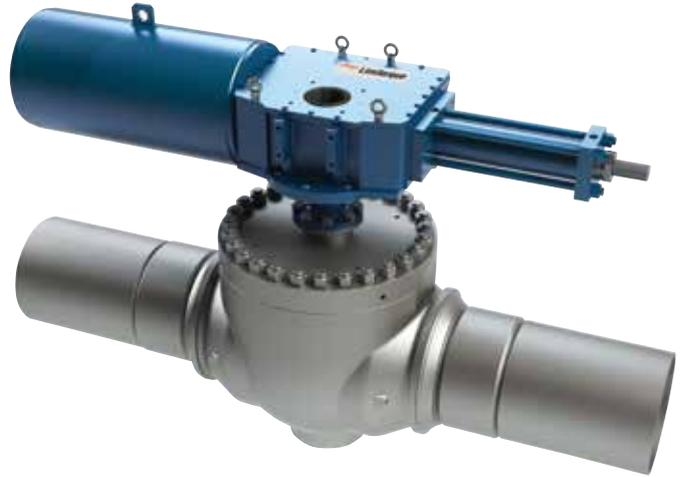
The LHS actuator features a 25-year design life, depending on service conditions, proper installation, operation and maintenance. In order to achieve this industry-leading design life, in-field maintenance is prescribed to be performed every six years of operation. For high-cycle applications, such as control valve operation, more frequent maintenance of replaceable wear surfaces, as outlined in EN 15714, may be required.
