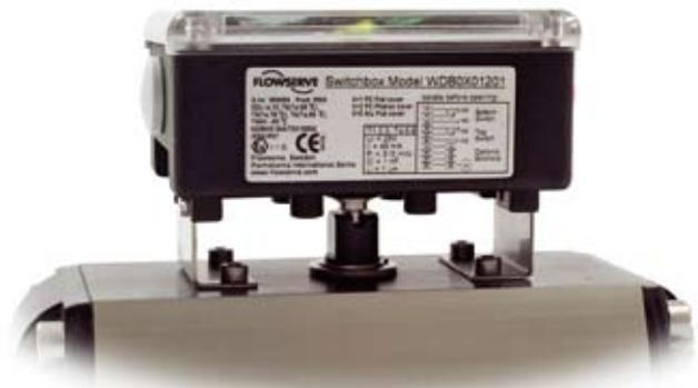
W series switchbox is designed to be directly and easily mounted onto actuators having connections according to Namur VDI/VDE 3845, in order to reduce switchbox/actuator overall dimensions. Picture shows W series with low profile mounting kit KL01.
