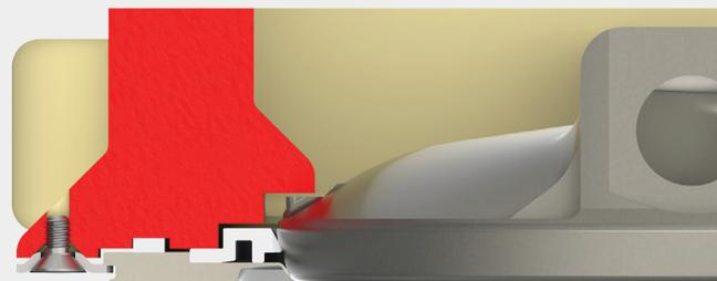
Figure 3: Dual fire-safe seating arrangement
